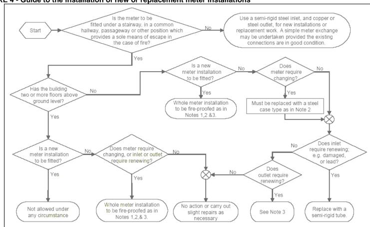
FIGURE 4 - Guide to the installation of new or replacement meter installations
