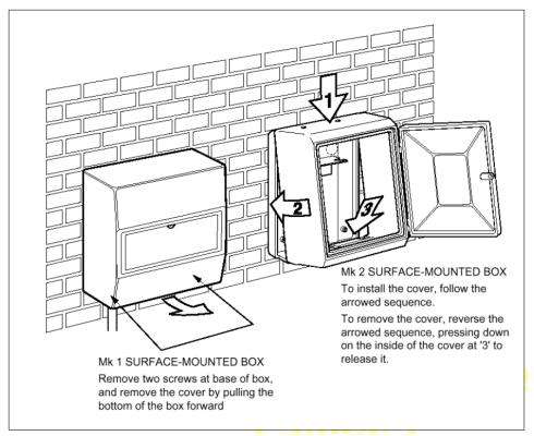
FIGURE 3 - Semi-concealed meter boxes (legacy installations only)
