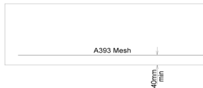
DETAIL SHOWING REINFORCEMENT ARRANGEMENT
