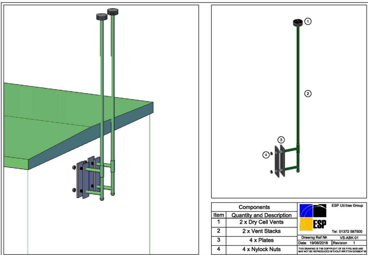
Type 'B' (See ESP/PL/PRI Vent Specification for Vent Stack Arrangement).
