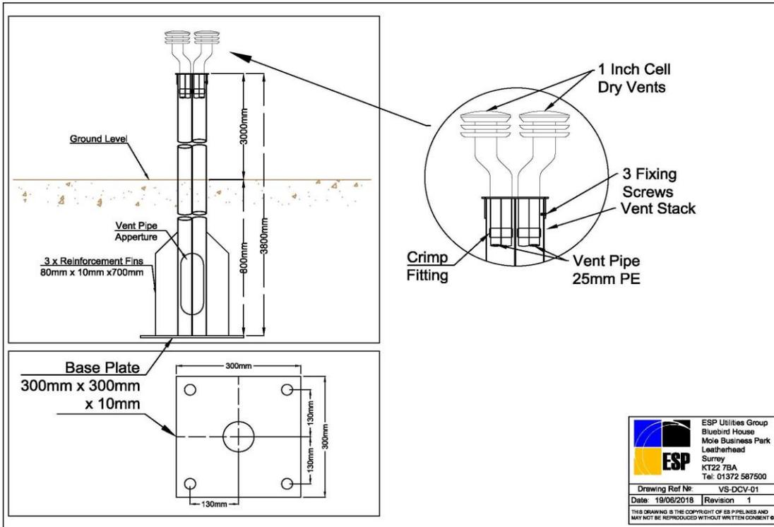
Standalone Vent Stack Base Construction and Dimensions for Type 'B'
